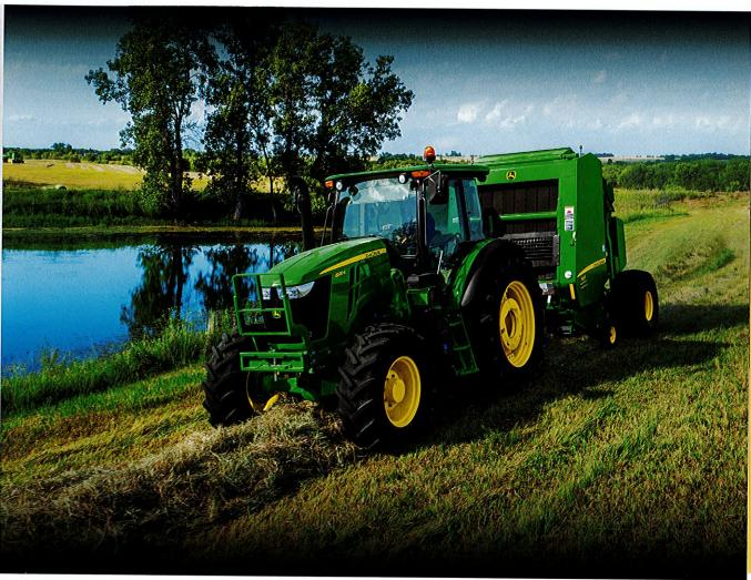
Get 11 speeds in the working range of 5 to 13 miles per hour (8 to 20 km/h) and a top transport speed of 25 mph (40 km/h) with the optional 24/12 transmission.
