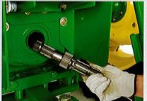
The 540/1000 rpm PTO shaft is easily reversible in less than 30 seconds because of the dry sump PTO housing.
