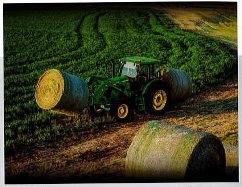
With 3,946 pounds (1789 kg) of lift capacity, an H Series Loader handles round bales ... and can even lift and stack two 5X6 bales easily.
