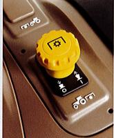
Engaging the PTO is an easy, smooth pushpull operation. And because the system is independent, stopping or downshifting the tractor won't change the PTO rpm levels.
