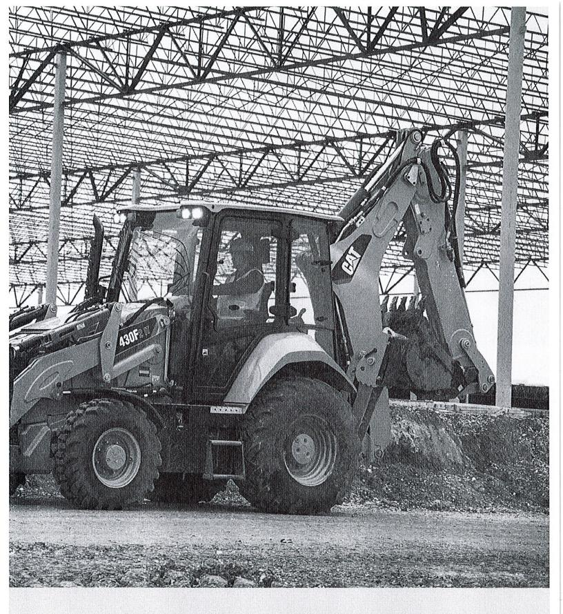
Experience the Backhoe Loader designed around customer feedback. The Cat 430F2 Backhoe Loader puts all the machine controls at the operator's fingertips. Operate all auxiliary controls with thumb rollers. Move from job site to job site quickly and smoothly with the additional 6th gear on the autoshift transmission and optional lock-up torque converter.
