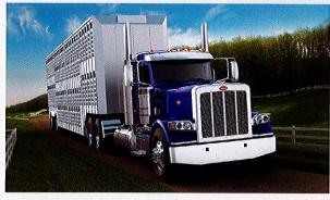
The Model 389 features conventional styling, plus a selection of components and options for efficiency and performance. Peterbilt's lightweight and durable hood is the industry's only all-aluminum hood with a distinctive punched oval grille and one-piece aluminum crown.
