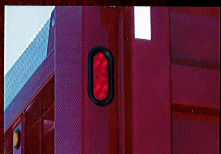
Recessed and rubber grommeted LED lighting.
