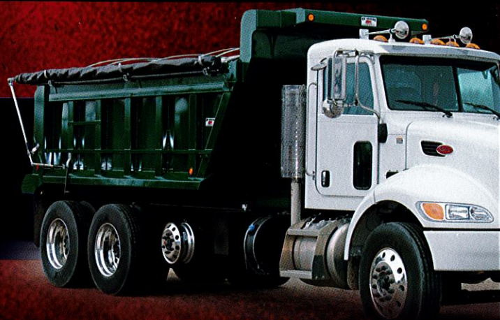
Optional Horizontal Side Rib & Sloped Tailgate
