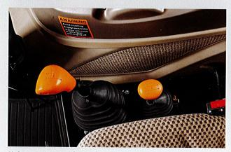
Shift on the fly: Don't stop to change gears. The 6E transmissions are synchrozed when shifting from B to C, C to D and D to C ranges
