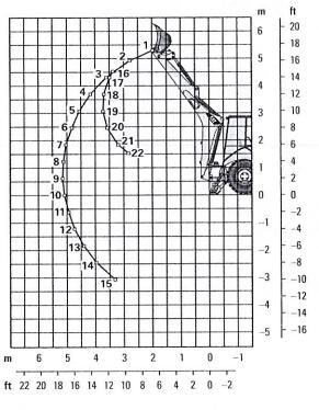
Lift capacities are over-end values calculated according to SAE J31. Values are 87% of the maximum lift force available. Machine equipped with AWD, OROPS, 0.96 m³ (1.25 yd³) general purpose bucket and 460 kg (1,015 lb) counterweight. Extendible stick includes 460 kg (1,015 lb) counterweight.
