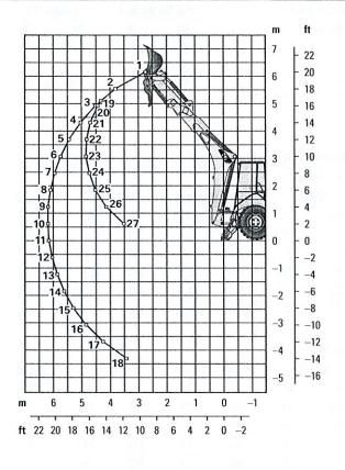
Lift capacities are over-end values calculated according to SAE J31. Values are 87% of the maximum lift force available. Machine equipped with AWD, OROPS, 0.96 m³ {1.25 yd³} general purpose bucket and 460 kg {1,015 lb} counterweight. Extendible stick includes 460 kg (1,015 lb} counterweight.
