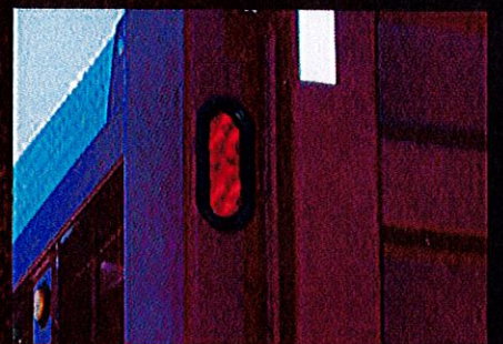
Recessed and rubber grommeted LED lighting.
