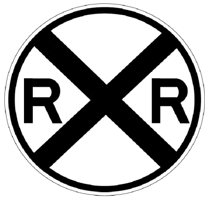
DETAILS OF RAILROAD ADVANCE WARNING SIGN ★ W10-1
