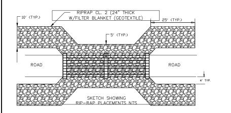
ABUT. 36 TONS/BENT 44 TONS
