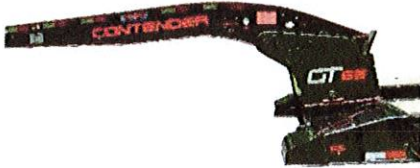
Low Profile Cantilever Neck. 45" above the deck. Plumbed for GN Extensions
