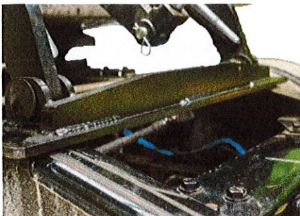
Self-Leveling Frame Jack Prevents Point Loading and the Need for Dunnage.
