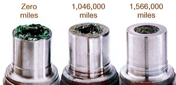
Real life examples of high mileage u-joints show virtually no wear
