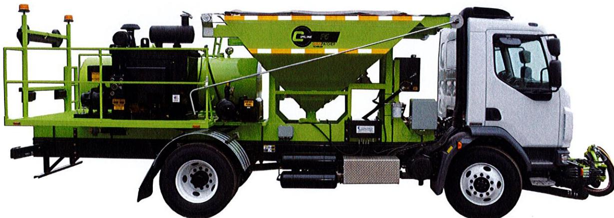
The covered five-yard aggregate hopper with vibrator feeds the venturi via dual air operated slide gates. The hopper is sized to allow 2 fills for every 1 fill of the emulsion tank.
