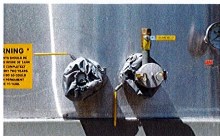
Dual Heated/Insulated Outlet Valves
