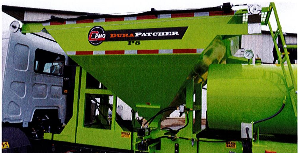
Dedicated diesel engine operates at pre-set low rpm and frees the truck engine to propel the vehicle.
